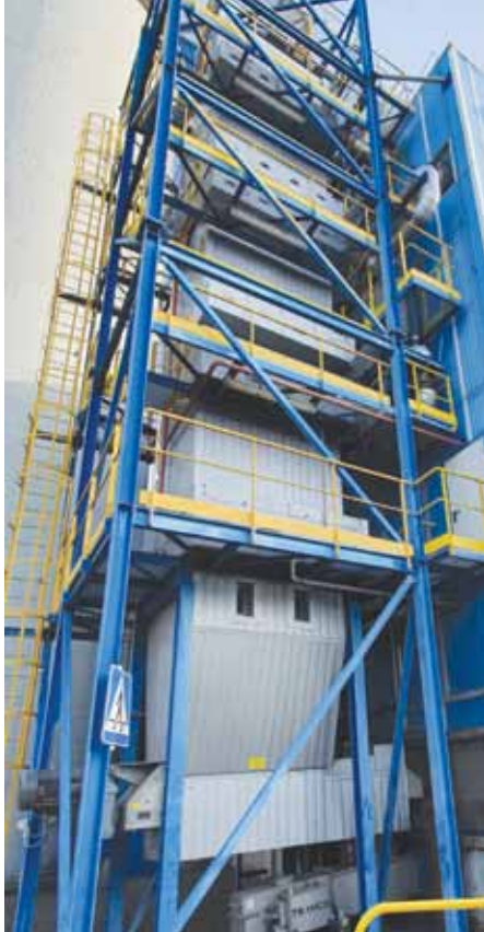
Vertical plate technology relies on conduction and not convection to cool potash, thereby minimizing emissions and reducing energy consumption. Photo courtesy of Solex Thermal Science.
